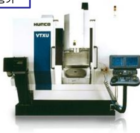
VTXU [수직 5축다면가공기 1대] Stroke(X,Y,Z) 800×698×508 C=360° A=-30°/+110°
